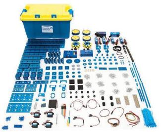
You'll also get a storage bin, an assortment of screws and nuts, tools, a 12V 3000 mAh NiMH battery pack, and a charger. Servos and high-resolution encoders are also included.
